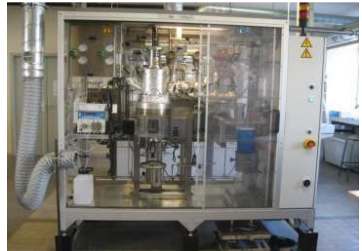
Pilot Reactor for Polyamides Synthesis (1L, 350°C, 50 bars)
