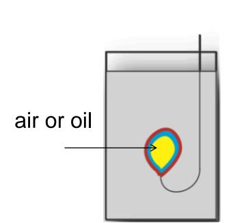
2. Compression of the droplets and pressure measurement to obtain interfacial tension as a function of area
