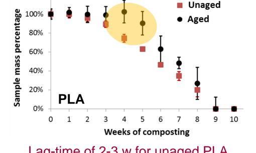
Lag-time of 2-3 w for unaged PLA and 3-4 w for aged PLA Complete biodegradation at week 9 for both
