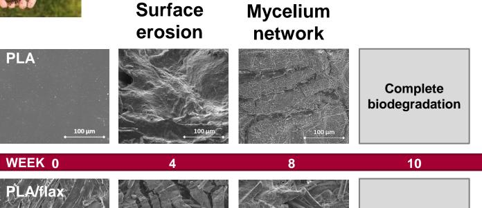
Complete piodegradation **Protrusion of the flax fibers**
