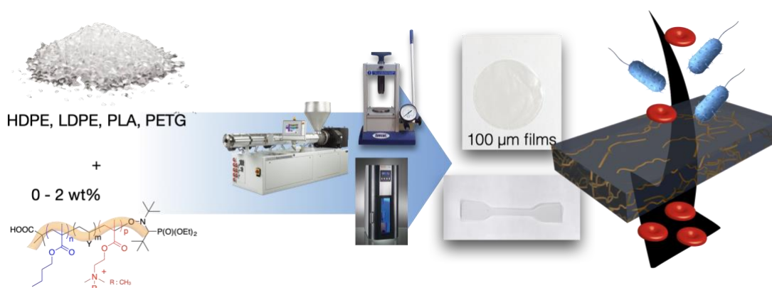
Figure 1. Elaboration of antimicrobial organic materials by co-extrusion with synthetic antimicrobial copolymer
